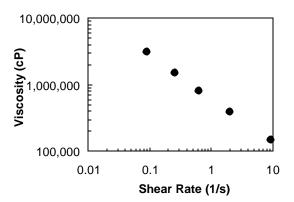
Viscosity measured by using the caulking viscometer (CV-100) for a caulking at  $24.2^{\circ}$ C
