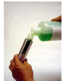
Fig.2 Pour the sample into the syringe up to the top of the viscometer main body.
